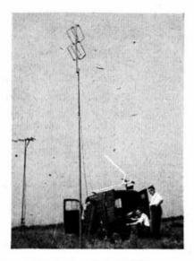
This view of G3APY/P, Alport Height (1,100 ft.), near Ambergate, Derbyshire, shows three of the aerial systems used during the 420 Mc/s. tests: a 5-element Yag; a "double quad" and a corner reflector. G3APY is at key while G8UZ keeps a wary eye on the photographer—G2AMD.
