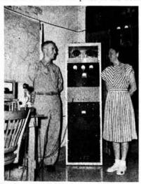
Many DX stations made their first contact with Honduras, Central America, as the result of the activities of Marion and Nan Brashear at HRIMB. The transmitter ends in a pair of 812's and runs at 150 watts input.
